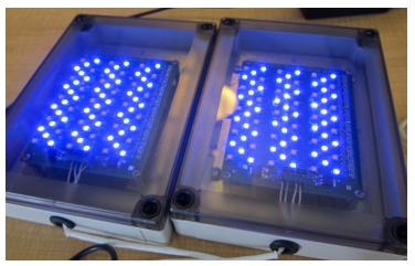
What started as a concept and parts purchased from a local Home Depot came to life. The Funk Engineering team selected the LEDs and designed a board to accept them. They had custom boards fabricated and then populated them with the LEDs. They also created a control box that would allow both light styles to be dimmed in and out alternatively or at the same time. Additionally, a power supply was included for the entire set up.
